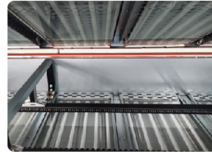
上下双向加热灯光, PCB板加热均匀 Top and bottom heating tube, PCB heated evenly.
