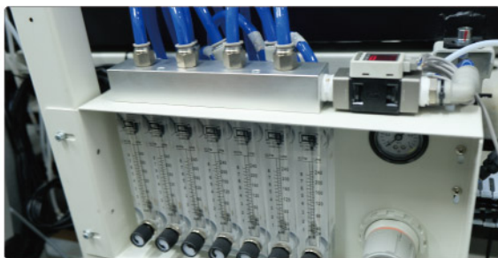
氮气保护系统, 氮气消耗量低 the oven adopts a full enclosed design which is to prevent the N 2 losing
