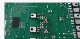
不能过波峰焊的双面PCB板 Double sided PCB board that cannot be soldered through wave soldering
