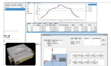
真空炉专用测试仪测试温度曲线 Profile tested by special profiler for vacuum reflow oven
