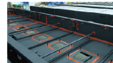
全密闭炉膛，耗氮少，残氧量低 Full closed furnace, low nitrogen consumption, low residual oxygen
