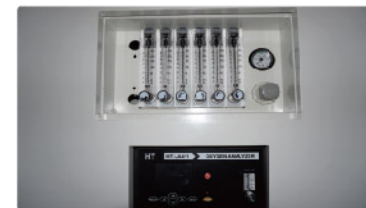
全程充氮，避免元器件氧化 N 2 filling in every zone to avoid components from oxidation in production process
